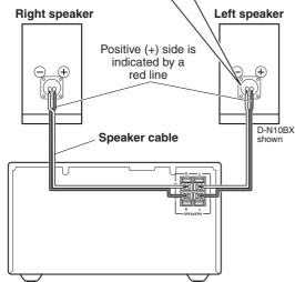
The type of speaker terminals used on the receiver and their position depends on the model. Refer to the receiver's instruction manual for details on connecting speakers to the receiver.
