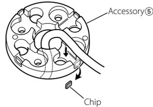
Break off the spacer chip in the direction where you want to wire the controller cable.
