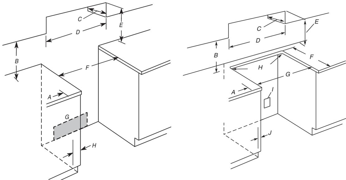
A. 4" (10.2 cm) min. clearance from both sides of range to side wall or other combustible material
