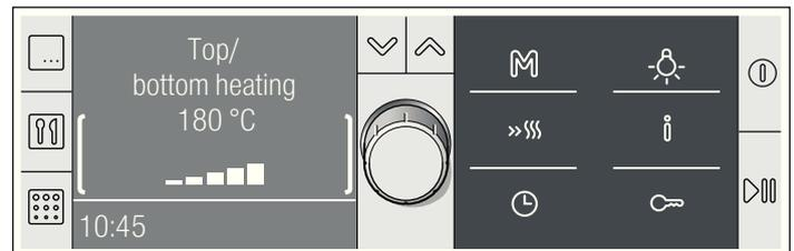
The bars do not appear when settings are made for grilling and cleaning.
