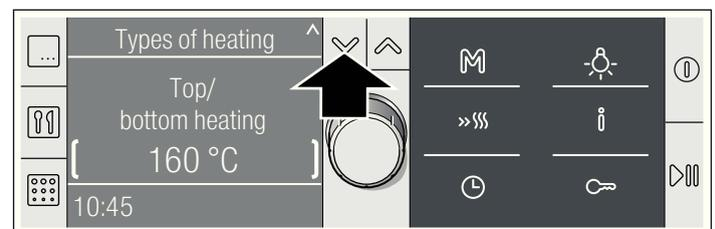
3. Turn the rotary selector to set the desired temperature.
