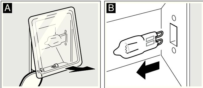
4. Refit the glass cover. Make sure that the curvature in the glass is on the right. Insert the glass at the top and push it in firmly at the bottom (Fig. C). The glass cover will click into place.
