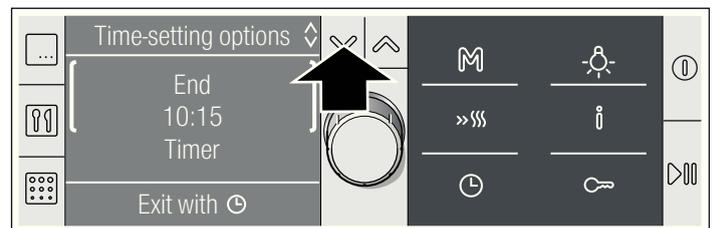
2. Set a later end time by turning the rotary selector.
