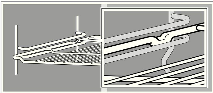
With the pull-out rails at level 2, you can pull the accessories out further.
