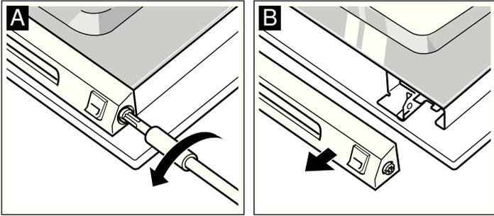
Make sure that the oven door is not closed while the cover is removed. The inner panel may be damaged.
