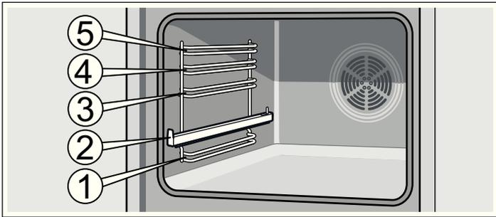
The accessories can be pulled out approximately halfway until they lock in place. This allows dishes to be removed easily.
