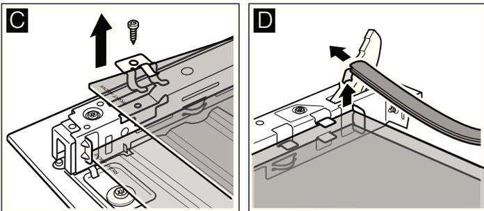
6. Pull the lower panel at an angle, upwards and out.
