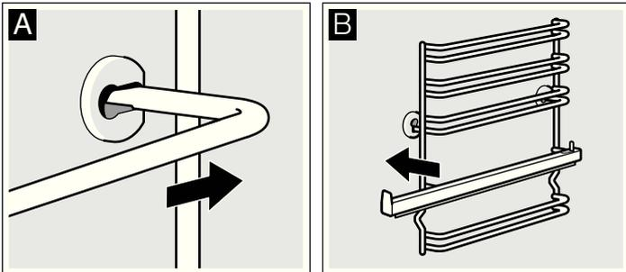
The rails only fit on the right or the left side. Ensure that, as shown in figure B, levels 1 and 2 are below and levels 3, 4 and 5 are above. The pull-out rail must be pulled out forwards.
