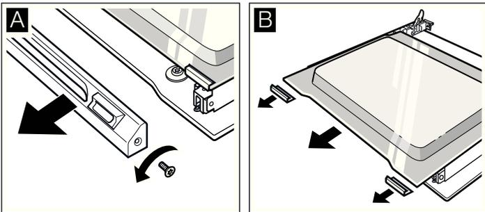
4. Unscrew the retaining clips on the right and left. Lift the panel and remove the clips from the panel (fig. C).
