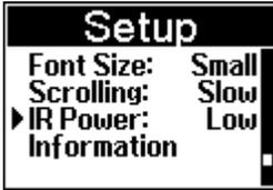
The M208 can send the IR commands with two different power levels. This offers you particular advantages if you frequently want to control devices over longer distances or if you have a device that doesn't react very sensitively to IR commands.
