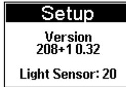
Additionally, this menu also displays the brightness values as calculated by the brightness sensor in the lower part of the remote control. This value can be between 0 and 255. 0 indicates complete darkness; 255 is the brightest value.
