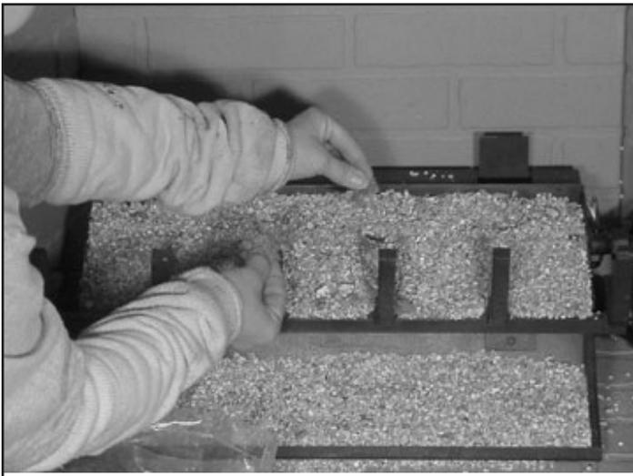
Figure 5 Placing Rock Wool
