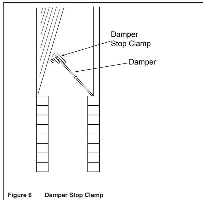
Figure 6 Damper Stop Clamp
