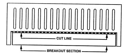
The breakout panel is removed by scoring the groove with a razor knife and bending the shaded portion away from the cut. The remaining edge can then be touched up with a small file. This allows the wiring to be run directly out of the control panel side of the amplifier.
