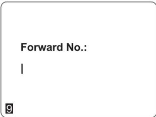
There will be a number 9 on the bottom left corner of the screen, indicating the current input mode. Press
