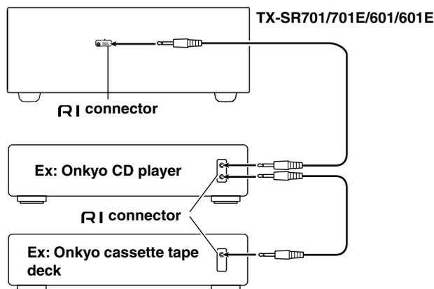
To connect components using the RI terminal, simply connect a remote control cable from this RI terminal to the RI terminal of the other component. An RI remote control cable with a 1/8-inch (3.5-mm) miniature two-conductor plug comes with every cassette tape deck, compact disc player, MD recorder, and DVD player that has an RI terminal.
