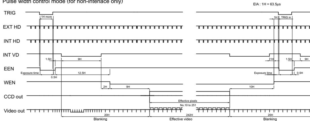
**CV-M50 CCIR (Non-interlaced / Field accumulation mode)**
