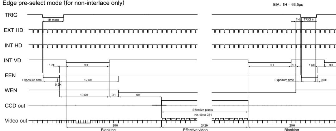
CV-M50 CCIR (Non-interlaced / Field accumulation mode)
