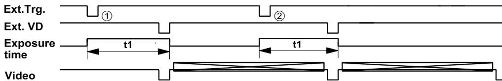
**b) 2:1 Interlaced mode (Field accumulation mode)**
