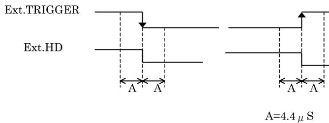
3. The ext. trigger input is 75 Ohm terminated as factory setting. (R127 short and SW2-2 ON). The voltage level of the ext. trigger has to be 4.0 Vp-p  $\pm$  2.0 V. The duration should be more than 1 H negative going. >64  $\mu$ sec. and < 60 msec. The input is AC coupled.
