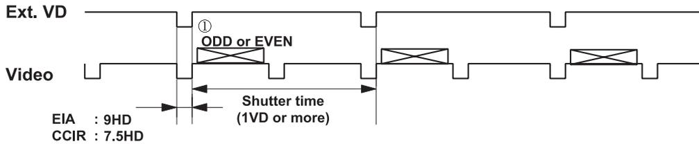
**b) 2:1 Interlaced mode (Frame accumulation mode)**
