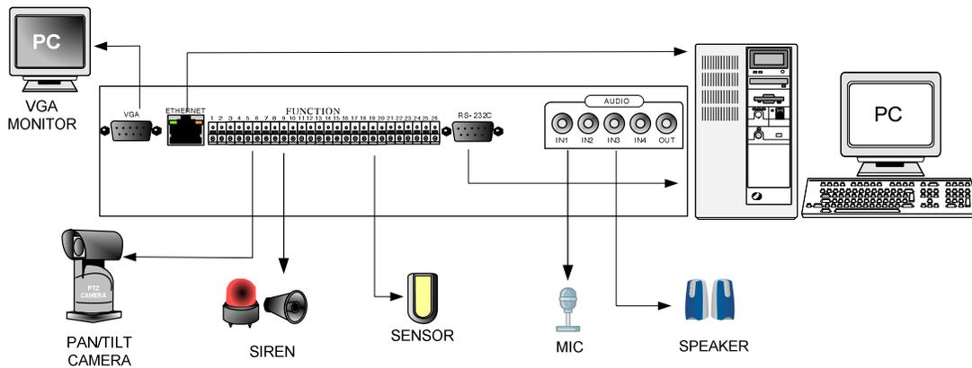
**RS-232C** : Control DVR through RS-232C port by using PC.
