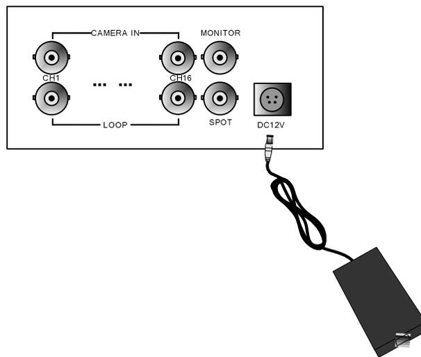
Connect one DC 12V, 6.67 A Adaptor to the back side of Power Jack for right operation of 2HDDs and CDRW.
