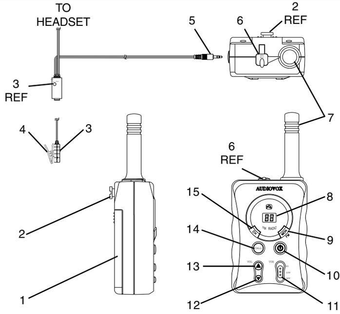
1. **Battery Compartment Cover:** Four (4) AAA batteries accessible when cover is removed.
