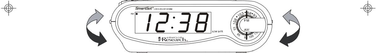
**FM** – The FM antenna is built in to the AC power cord. If FM reception is weak try varying the position and direction of the power cord until you find the strongest signal.
