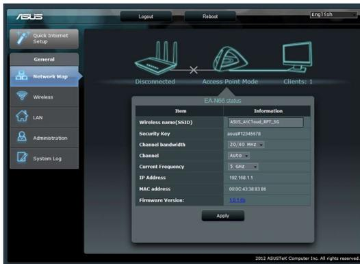
On the left side of the screen is the Advanced Setup panel. Use the Setup panel to navigate to specific features of the EA-N66.
