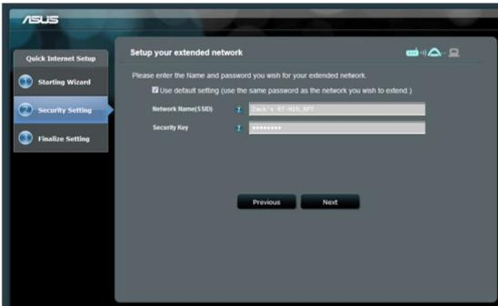
By default, the EA-N66 will assign an SSID using the following format: **"original-SSID\_RPT"**.
