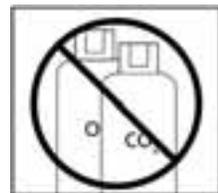
USE COMBUSTIBLE GASSES OR ANY OTHER REACTIVE GAS AS A POWER SOURCE FOR THIS NAILER/STAPLER. Explosion and serious personal injury could occur.
