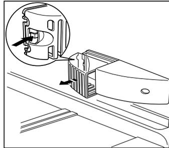
press on the rear hook and at the same time slide the cover in the direction indicated by the arrow.
