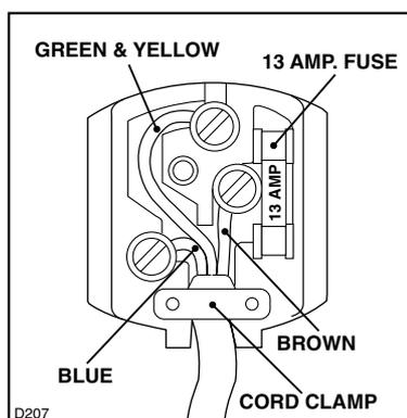
1. Connect the Green and Yellow (earth) wire to the terminal in the plug which is marked with the letter «E» or the earth symbol  $\oplus$  or coloured green and yellow.
