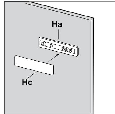
Open the appliance door and the furniture door at 90°. Insert the small square (Hb) into guide (Ha). Put together the appliance door and the furniture door and mark the holes as indicated in the figure.
