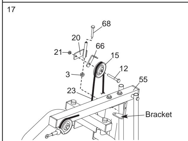
Properly tighten the 5/16” x 5” Bolt (68) and a 5/16” Nylon Locknut (3) attaching the Pulley Bracket (20) to the bracket on the Top Frame (55). **Do not overtighten the Locknut; the Pulley Bracket must be able to pivot easily.**
