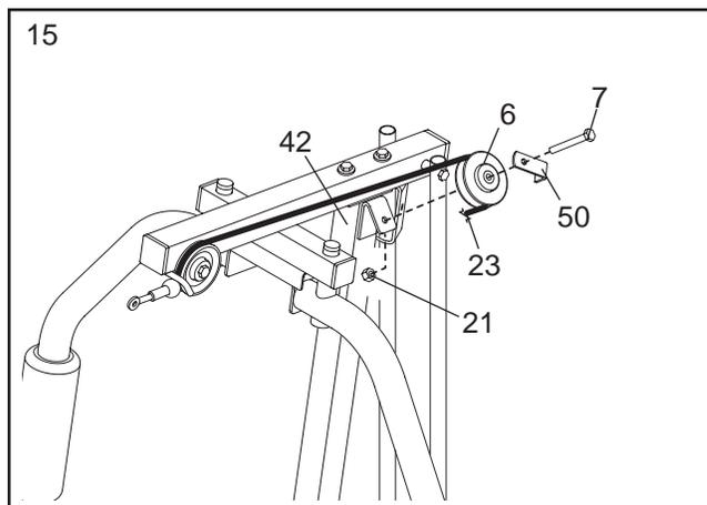
16. Route the Long Cable (23) around a “V”-pulley (6). Attach the “V”-pulley and a Long Cable Trap (50) to the Left Arm (47) with a 3/8” x 2 1/2” Bolt (7) and a 3/8” Nylon Locknuts (21). **Make sure that the Long Cable Trap is positioned to hold the Cable in the groove of the “V”-pulley.**
