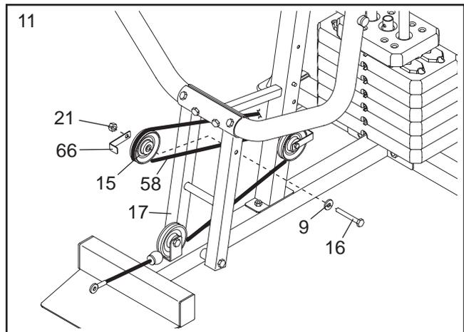
12. Route the Short Cable (58) under a 3 1/2" Pulley (15). Attach the Pulley and a Cable Trap (66) to the upper hole in the Front Upright (42) with a 3/8" x 3 3/4" Bolt (71), a 3/8" Washer (9), and a 3/8" Nylon Locknut (21). **Make sure that the Cable Trap is turned to hold the Cable in the groove of the Pulley.**
