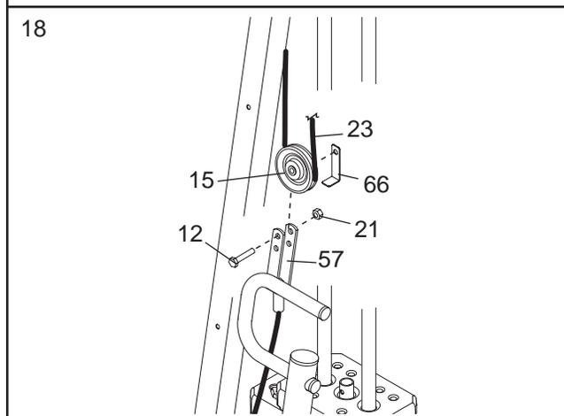
19. **Note: The 3 1/2" Pulley (15) in this step has been preassembled. It is shown exploded in this drawing for clarity.**
