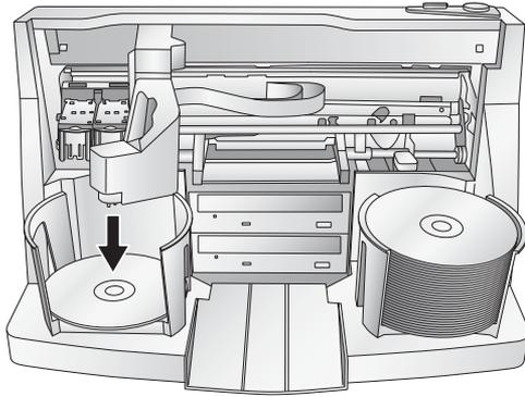
9. The Robotic Disc Transporter will now load the second recorded disc of the first round into the Printer Tray for printing.
