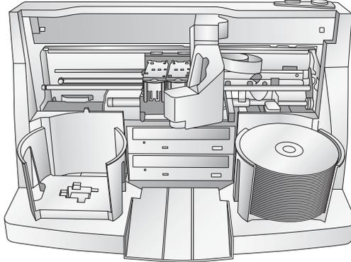
2. The Publisher's integrated Robotic Disc Transporter will first check your recorder drives for a disc by attempting to "pick" from the recorder. Then, the Robotic Disc Transporter will pick a disc from the Input Bin.
