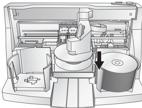
4. The Recorder Trays then automatically shut. As soon as each drive tray closes the burn process will begin for that drive. With two drives, each drive burns independently of the other. If a disc does not record properly (meaning that all or part of that disc is not recordable), the Robotic Disc Transporter picks it out of the Recorder Tray and sends it to the Reject Area.
