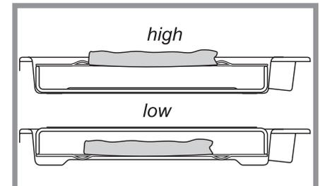
**7** The grill pan grid can be turned over to give two grilling positions.
