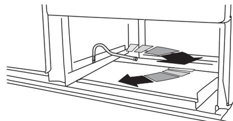
*Turn the levelling tool clockwise, two full (180°) turns. It will be stiff. The front of the oven will rise slightly as the roller drops down.*
