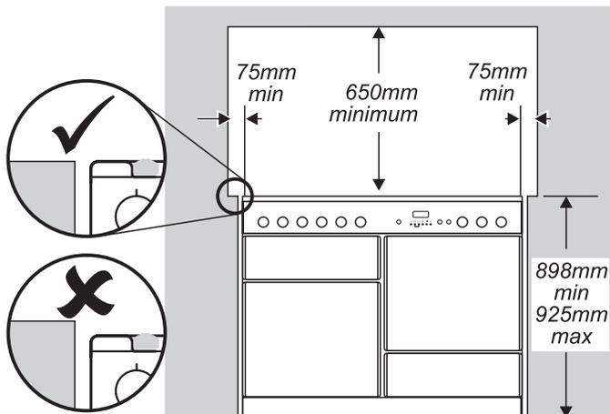
The hotplate surround should be level with, or above, any adjacent work surface. Above hotplate level a gap of 75mm should be left between each side of the cooker and any adjacent vertical surface.
