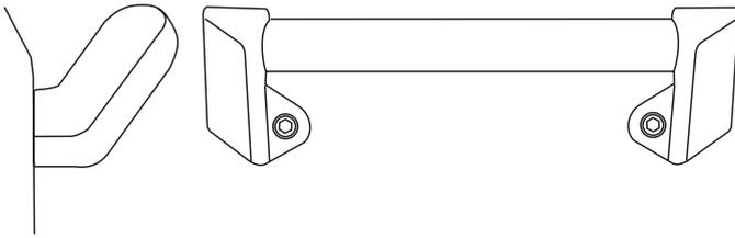
Remove the 4mm Allen screws from the top corners of the fascia and fix the front handrail in position.
