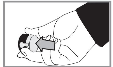
If when you let go of the control knob the burner goes out, the safety device has not held in. Turn off the grill and wait one minute then try again this time holding in the button for slightly longer.
