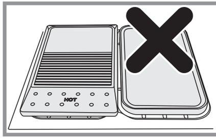
**5** Always leave space around the griddle for the gases to escape. **Never** fit two griddles side by side. Large pans should also be spaced well apart. The maximum pan base diameter is 250mm (10in).
