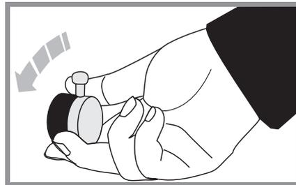
**4** The grill has a special safety device with stops the flow of gas to the grill if the flame goes out. Turn the knob to the large flame symbol (♠). Press in the grill knob. This lets gas through to the burner. Keep holding the knob pressed in and press the igniter button or light with a match. Keep holding the button for about 10 seconds
