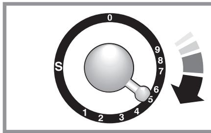
**2** Turn the control knob back to the Mark you wish to cook on and for best results pre-heat the oven for 15 minutes before placing your dishes in it.
