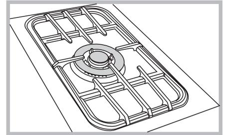
**4** Simmering aids, such as asbestos or mesh mats, are NOT recommended. They will reduce burner performance and could damage the pan supports.
