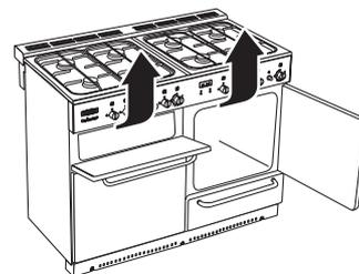
Open the grill door and right hand oven door so that you can get a good grip on the bottom of the fascia panel as you move the oven.
