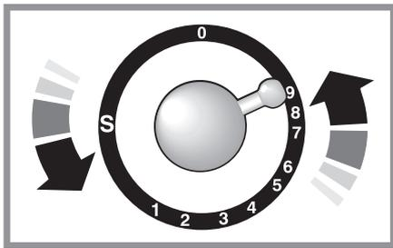
**1** Push in and turn the knob controlling the oven to Gas Mark 9. The oven will light automatically.
