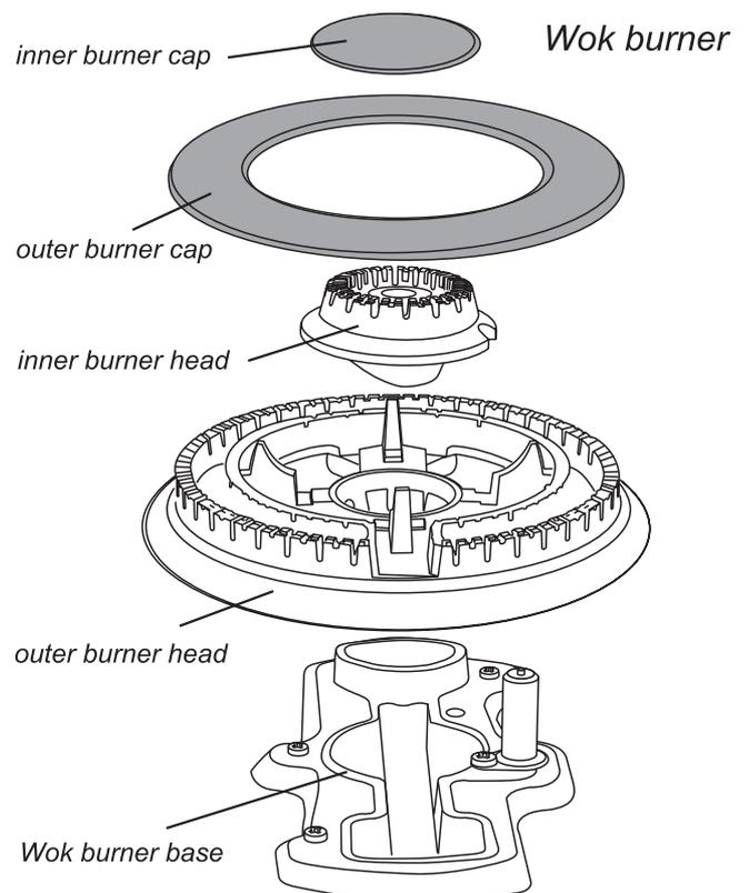
When reassembling the Wok burner, turn over the large base ring and find the 'D' shaped area.
