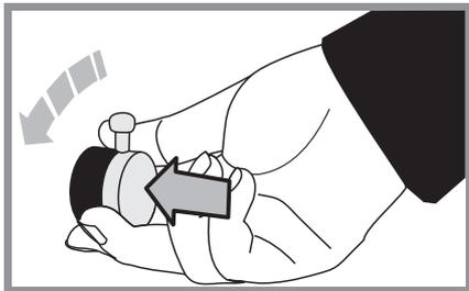
**4** Press in the grill knob, turn to the large flame symbol (♠) and press the igniter button or light with a match.
