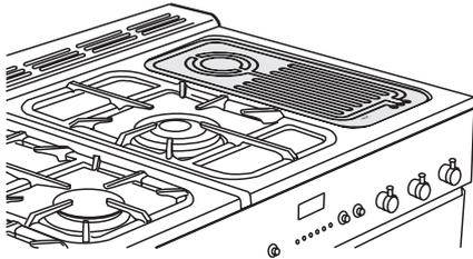
Use the warmer for keeping food warm while the final touches are put to a meal. Turn the control knob anti-clockwise to the 'On' position. The 'HOT' indicator lights up. For best results, pre-heat a covered serving dish for 10 minutes before adding food to it.
