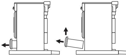
Fit the levelling tool on the rectangular adjuster as shown below.
