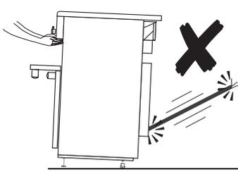
*If a stability chain is fitted, release it as you ease the cooker out.*
