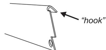
When refitting make sure that the trim is in the middle of the front of the oven burner bracket.
