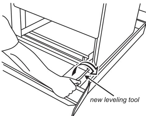
Make sure you lower **BOTH REAR ROLLERS**. There are two adjusting nuts, one for each roller, at both the front bottom corners of the cooker.
