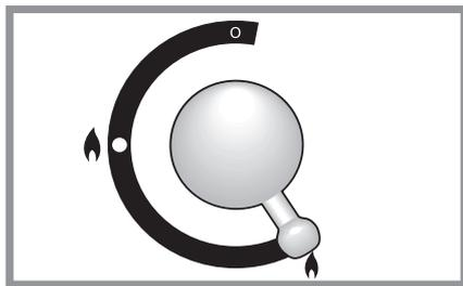
**5** The low position, marked with the small flame symbol, is beyond high, not between high and off.
