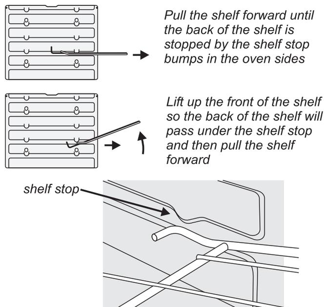
To refit the shelf, line up the shelf with a groove in the oven side and push the shelf back until the ends hit the shelf stop. Lift up the front so the shelf ends clear the shelf stops, and then lower the front so that the shelf is level and push it fully back.
