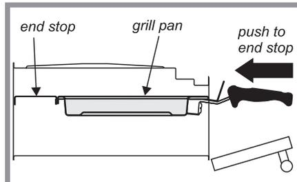
**6** For best results preheat for 2 minutes with the grill pan in position. After placing your food on the grill pan grid, slide the grill pan onto the side supports just below the burners. Adjust the flame height to suit by turning the knob.
