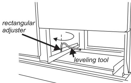
**LOWER THE FRONT ROLLER** by doing 14 complete (360°) turns clockwise. (This means turning and removing the levelling tool 56 times).
