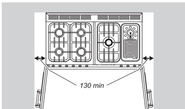
A clearance of 130mm is required if the cooker is near a corner of the kitchen to allow the oven doors to open.
