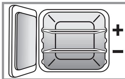
**5** Dishes placed above the central position will be cooked at approximately one gas Mark higher, dishes cooked below approximately one gas Mark lower. You can therefore cook dishes requiring different gas Marks at the same time.
