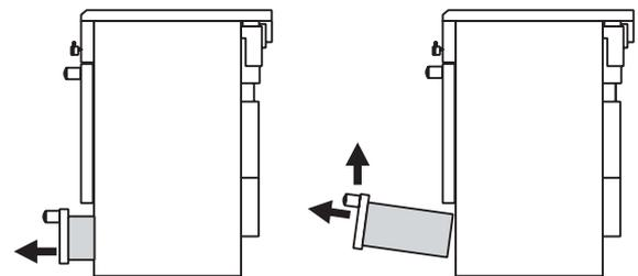
Your installer may not have left the levelling tool in place. If not, locate it as shown. If you cannot find the levelling tool, contact your installer.
