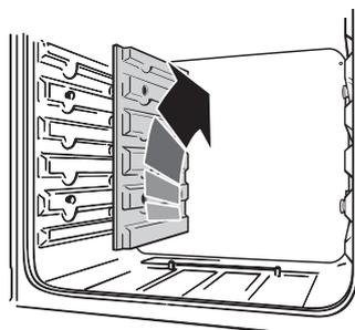
Each side of the oven is fixed with four fixing screws. You don't have to remove the screws to remove the oven linings. Lift each side panel upwards and they will slide off the screws. Then pull them forwards.
