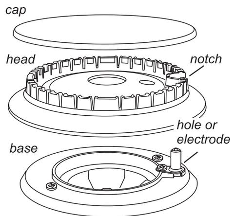
When refitting the burner head, make sure that the notch lines up with the electrode or hole in the base. Check that the burner head is level and that the cap is fitted centrally on the burner head.
