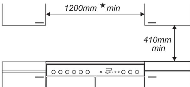
\*Any cooker hood should be installed in accordance with the hood manufacturer's instructions.
