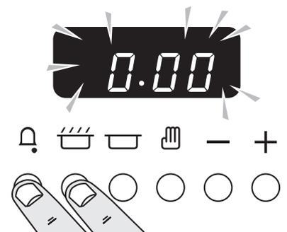
*Press and hold as above. At the same time, press (-) or (+) until the correct time shows. Don't forget it's a 24 hour clock. If you make a mistake or press the wrong button, turn off the power supply for a minute or two and start again.*
