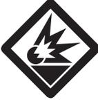
**Never connect to an air source that is capable of exceeding 90 PSI.** Over pressurizing the tool may cause bursting, abnormal operation, breakage of the tool or serious injury to persons. Use only clean, dry, regulated compressed air at the rated pressure or within the rated pressure range as marked on the tool. Always verify prior to using the tool that the air source has been adjusted to the rated air pressure or within the rated air-pressure range.
