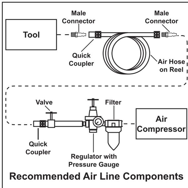
1. Incorporate an in-line oiler, shut-off valve, regulator with pressure gauge, and filter for best service, as shown in
