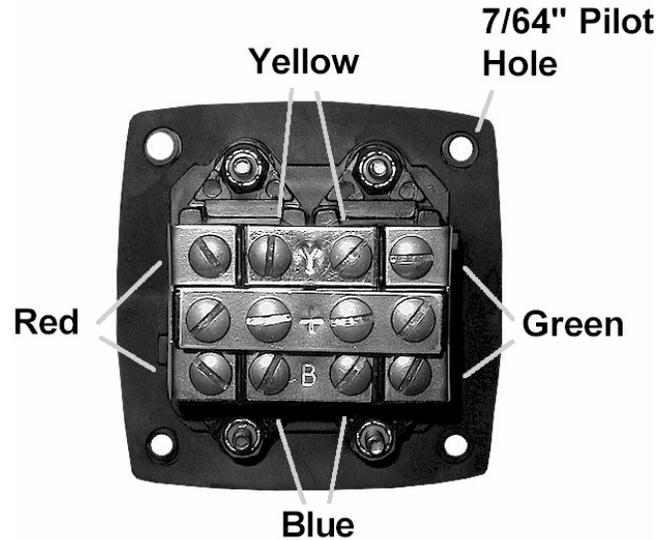
5. Mark the four locations for the 7/64" pilot holes and drill. Test fastening with the #8 screws. Open the holes to 1/8" if necessary.
