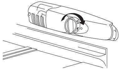
The temperatures in the refrigerator compartment and freezer compartment cannot be independently regulated.
