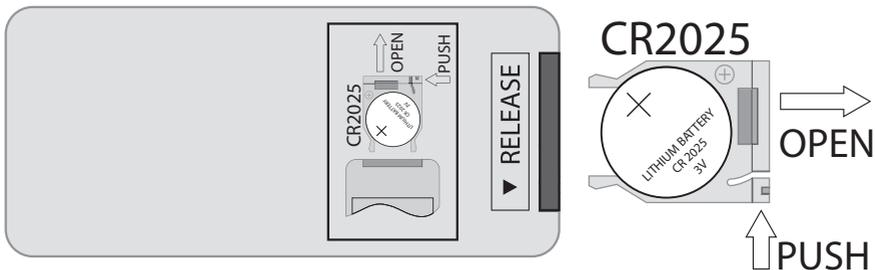
1. Push the Release Button and pull out the Battery Compartment to access the battery.
