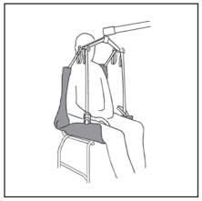
For closed leg positions, straps may be crossed under both legs and attached as shown. Ensure leg straps C and D are passed through straps A and B and attached to the spreader bar. This can provide additional comfort and can be used for some amputees.
