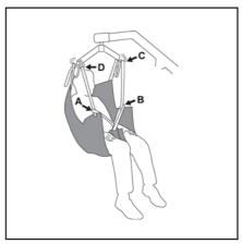
Check the sling is smooth under the pateient and the position is comfortable. Move the hoist into position and attach the leg straps to the spreader bar using the coloured loops. This maintains the patient in an upright sitting position. The lift may move towards the patient as you do this. When reseating the patient the hand grips may be used to ensure a good posture.
