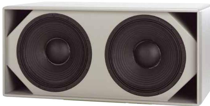
The AQ215 is a dual driver, direct radiating sub-bass in a heavily braced vented enclosure. It features two very efficient 15" (380mm) long-throw bass drivers with high power 4" (100mm) voice coils and generously sized low frequency ports for low noise, high power operation.
