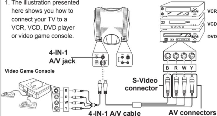
2. The cables are color-coded (black, red, white, and yellow). Connect each color-coded cable to the appropriate connector on your device.
