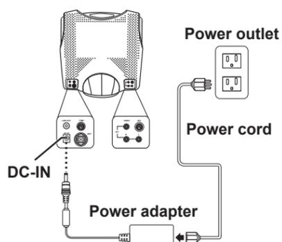
1. Connect the power cord to the power adapter as illustrated.
