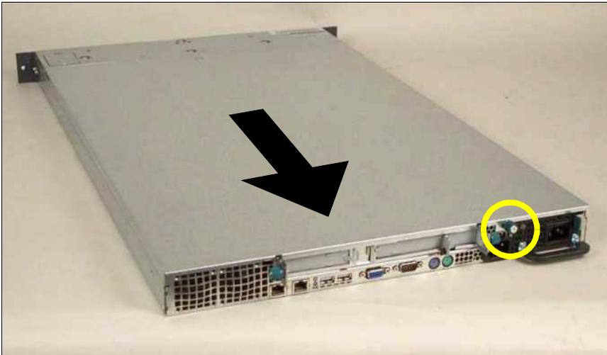
Figure 3: Removing the cover
