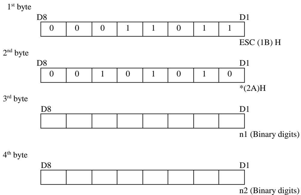
Bit image mode printing is performed by this command. (n2 is the equotient when divided by 256, and n1 is the remainder.) When data is received only for numbers specified by n1 and n2, printing and line feed are carried out automatically, and the bit image mode is cancelled.
