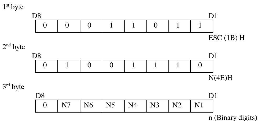
This command feeds the paper (skips) “n” lines without any printing. However, this cannot exceed the length of one page. ( $1 \leq n \leq 126$ )
