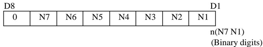
When the number of lines to be fed (2<sup>nd</sup> byte) is written-in following the paper feed command (1<sup>st</sup> byte), the paper will be fed by the number of lines specified. The number of lines to be fed can be specified from n = 1 to 127. If “0” is specified, paper feed will not be carried out.
