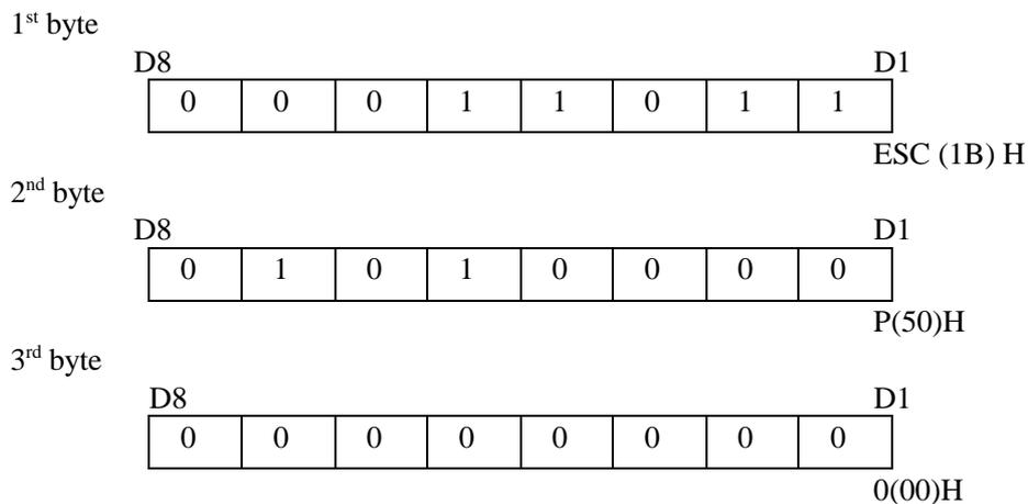
A full cut the paper is performed by this command (one connecting point remaining).
