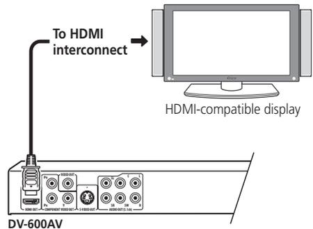
The arrow on the cable connector body should be face up for correct alignment with the connector on the player.
