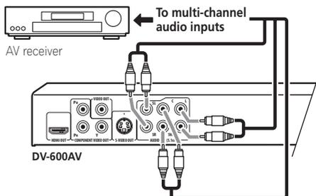
You can also use the SCART AV connector, the S-video (*DV-600AV only*) or component video jacks to connect to the AV receiver if you prefer.
