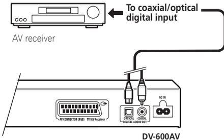
*DV-600AV only:* For an optical connection, use an optical cable (not supplied) to connect the **OPTICAL DIGITAL AUDIO OUT** jack to an optical input on your AV receiver.
