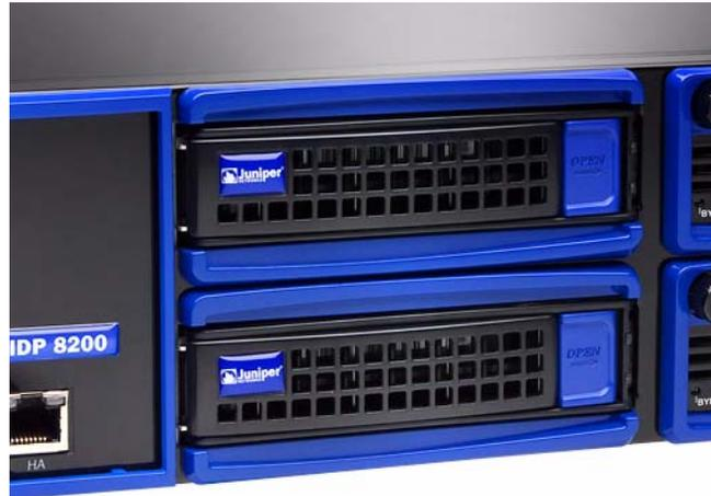
3. Press and hold down the latch to release the handle, and then pull the handle open.
