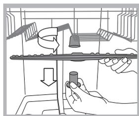
To remove the upper sprayer arm, turn the plastic locking ring in an anti-clockwise direction. The upper sprayer arm should be replaced so that the side with the greater number of holes is facing upwards.
