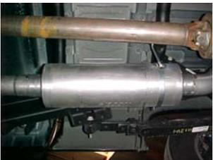
INSTALL MUFFLER # B ONTO HEAD PIPE #A 1-1/2" TO 2" WITH THE LOUVERS FACING TOWARDS THE CONVERTER. USE A JACK STAND TO SUPPORT THE MUFFLER. USE CLAMP #G SECURE THE MUFFLER TO THE HEAD PIPE. DO NOT TIGHTEN. MUFFLER INLET IS LOOKING INTO THE LOUVERS.
