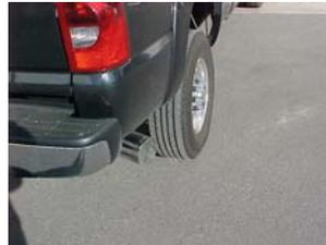
INSTALL STAINLESS STEEL TIP. CLAMP DOWN. WHEN YOU HAVE EVERYTHING IN PLACE, FIRMLY TIGHTEN ALL BOLTS AND CLAMP DOWN SECURELY. TO CLEAN STAINLESS STEEL TIPS USE ANY SAINLESS STEEL CLEANER AND SCOTCH BRITE PAD.
