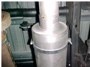
INSTALL BAND CLAMP #H ONTO MUFFLER. INSERT WELDED HANGER INTO RUBBER GROMMET. TIGHTEN BAND CLAMP USING HARDWARE KIT #I.
