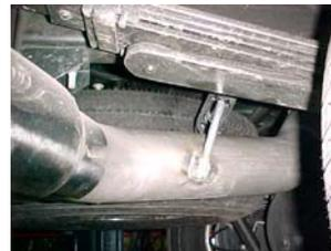
INSTALL THE TURNOUT PIPE #D ON TO THE TAILPIPE. SECURE TOGETHER WITH CLAMP #G. DO NOT TIGHTEN. ROLL THE EXIT PIPE UNTIL IT IS AT THE CORRECT ANGLE FOR YOUR TRUCK. INSERT WELDED HANGER INTO GROMMET.
