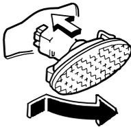
4. Install the new side turn signal unit in the reverse order of removal.
