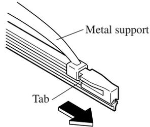
3. Remove the metal stiffener from each blade rubber and install them in the new blade.
