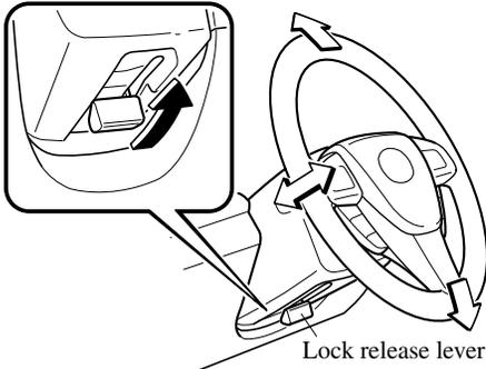
2. Tilt the steering wheel and/or adjust the steering column length to the desired positions, push the lever down to lock the column.
