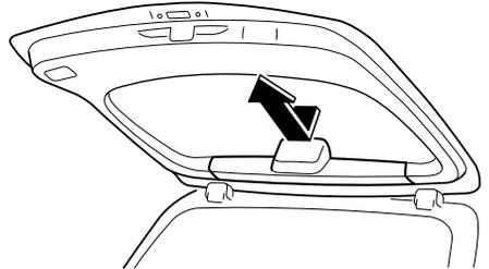
3. Disconnect the electrical connector from the socket.
