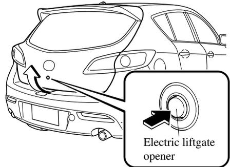
While the ignition is switched ON, the liftgate can be opened only when the vehicle is stopped with the parking brake applied (manual transaxle), or with the selector lever in the P position (automatic transaxle).
