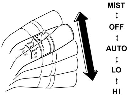
Turn the wipers on by pulling the lever down.
