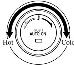
This dial controls temperature. Turn it clockwise for hot and counterclockwise for cold.
