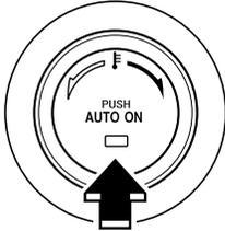
By pressing the AUTO switch the following functions will be automatically controlled in accordance with the selected set temperature:
