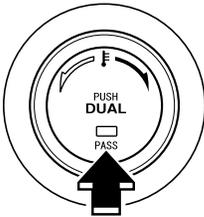
Use the DUAL switch to change the mode between the individual operation (driver and passenger) and interconnection modes.
