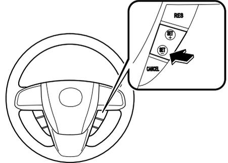
Your vehicle has a tap-down feature that allows you to decrease your current speed in decrements of 1.6 km/h (1 mph) by a momentary tap of the SET- switch. Multiple taps will decrease your vehicle speed 1.6 km/h (1 mph) for each tap.
