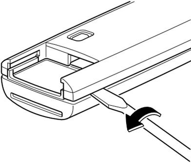
4. Remove the battery cap, then remove the battery.
