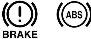
If the electronic brake force distribution control unit determines that some components are operating incorrectly, the control unit may illuminate the brake system warning light and the ABS warning light on simultaneously. The problem is likely to be the electronic brake force distribution system.
