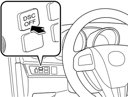
Press the switch again to turn the TCS/DSC back on. The DSC OFF indicator light will go out.
