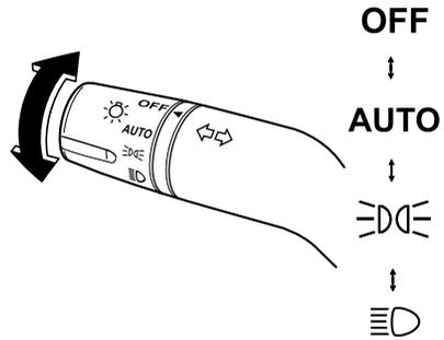
Turn the headlight switch to turn the headlights, other exterior lights and dashboard illumination on or off.
