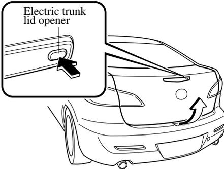
While the ignition is switched ON, the liftgate/trunk lid can be opened only when the vehicle is stopped with the parking brake applied (manual transaxle), or with the selector lever in the P position (automatic transaxle).
