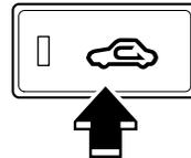
This switch controls the source of air entering the vehicle.
