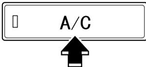
Press the A/C switch to turn the air conditioner on. The indicator light on the switch will illuminate when the fan control dial is set at position 1, 2, 3, or 4.
