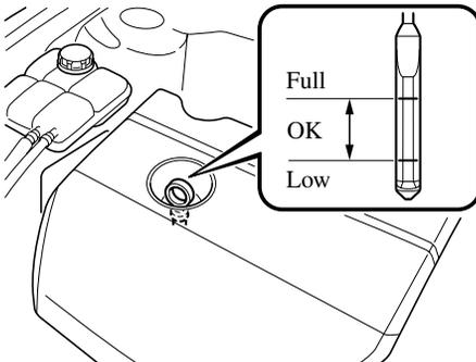
5. Pull it out again and examine the level. It's OK between Low or MIN and Full or MAX. But if it's near or below Low or MIN, add enough oil to bring the level to Full or MAX.
