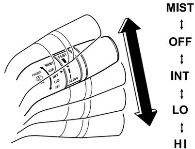
Turn the wipers on by pulling the lever down.
