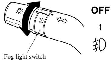
To turn them off, rotate the fog light switch to the OFF position or turn the headlight switch to the OFF position.
