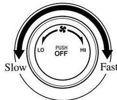
The fan has seven speeds. The selected speed will be displayed.
