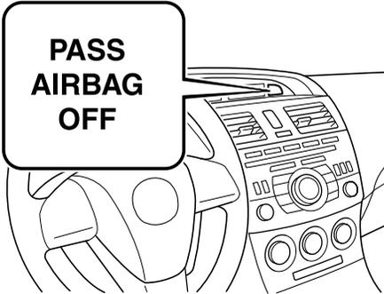
If the front passenger weight sensors are normal, the indicator light illuminates when the ignition switch is turned to the ON position. For a specified of time it goes out.
