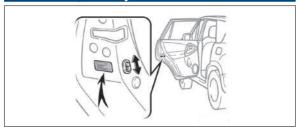
Move the lever to "LOCK," allowing the door to be opened only from the outside.
