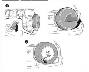
To remove the spare tire cover,\* open the back door. Unhook the latch on the bottom of the cover. After closing the back door, remove the cover.
