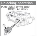
**NOTE:** After unlocking, if a door is not opened within thirty (30) seconds, all doors will relock for safety.
