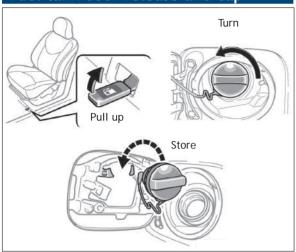
**NOTE:** If the cap is not tightened enough, the Check Engine " \( \sum\_{n} \)" indicator may illuminate.
