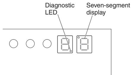
Figure 72. Numeric display LEDs
