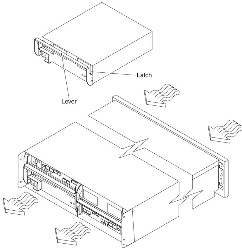
Figure 6. Power supply and fan unit and airflow
