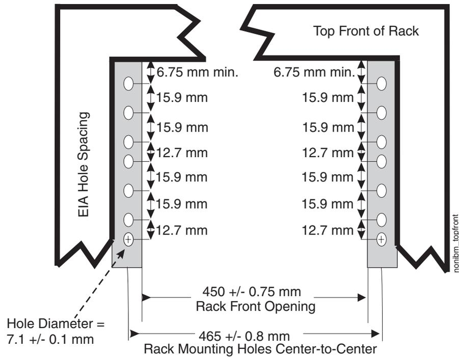
Figure 92. Rack specifications dimensions, top front view
