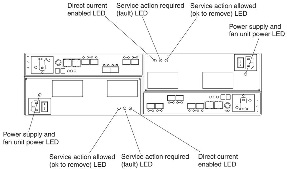
Figure 66. Power supply and fan unit LEDs
