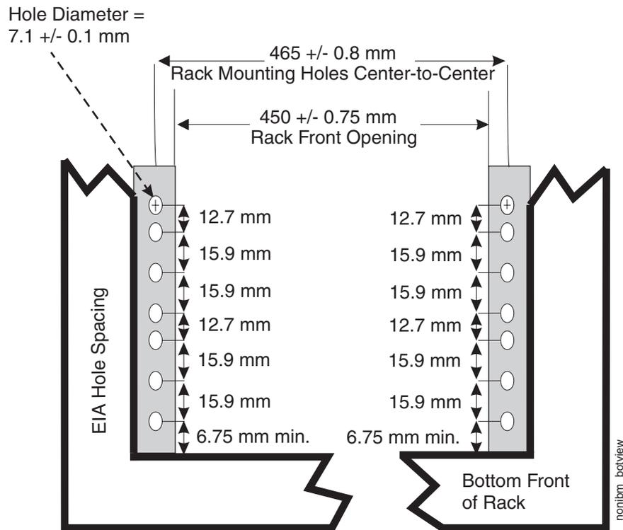
Figure 93. Rack specifications dimensions, bottom front view
