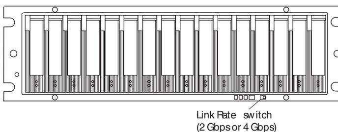
Figure 82. Link rate switch
