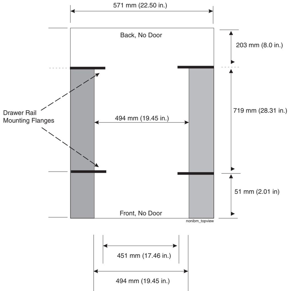
Figure 91. Top View of non-IBM Rack Specifications Dimensions
