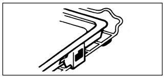
To check the progress of the food being grilled, the grill pan should be withdrawn on the shelf to tend the food during cooking, or the carrier shelf can be lifted away from the cooker and rested on a heat resistant work surface.
