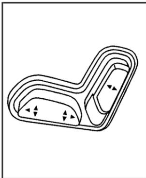
If the vehicle has power seats, the controls used to operate them are located on the outboard side of the seats.
