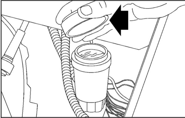
Refer to the Maintenance Schedule to determine how often to check the fluid level in the clutch master cylinder reservoir and for the proper fluid. See *Recommended Fluids and Lubricants* on page 6-11.
