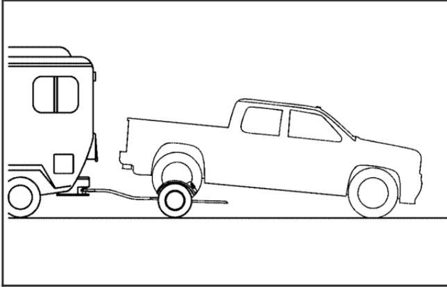
Use the following procedure to dolly tow a two-wheel-drive vehicle from the rear:
