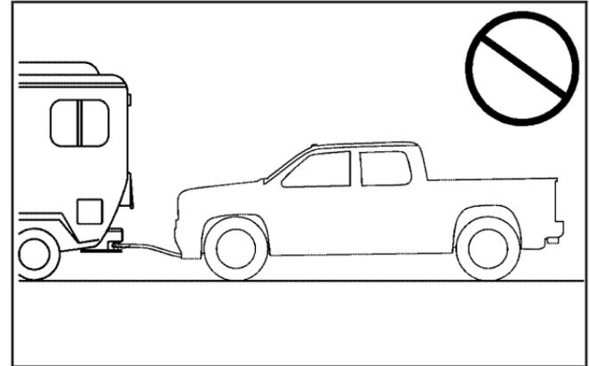
**Notice:** If the vehicle is towed with all four wheels on the ground, the drivetrain components could be damaged. The repairs would not be covered by the vehicle warranty. Do not tow the vehicle with all four wheels on the ground.
