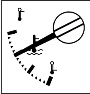
This gage shows the engine coolant temperature.
