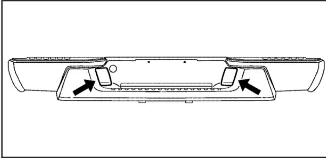
1. Reach under the rear bumper for the bulb socket.
