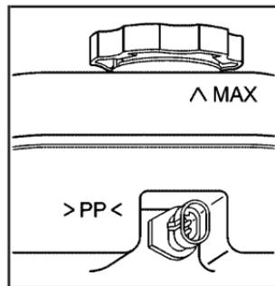
The fluid level should be above the PP mark. If it is not, have the brake hydraulic system checked to see if there is a leak.
