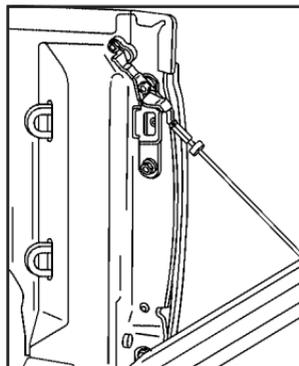
2. Remove the retaining cable from the passenger side of the tailgate by pulling the clip away from the bolt head while pushing the cable bracket forward. When the larger part of the hole on the bracket is over the bolt, slide the bracket off of the bolt.
