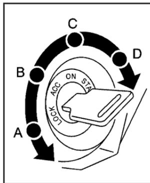
The ignition switch has four different positions.
