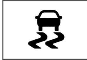
The StabiliTrak and Traction Control System (TCS) indicator/warning light comes on briefly while starting the engine.
