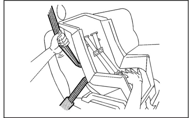
7. To tighten the belt, push down on the child restraint, pull the shoulder portion of the belt to tighten the lap portion of the belt and feed the shoulder belt back into the retractor. When installing a forward-facing child restraint, it might be helpful to use your knee to push down on the child restraint as you tighten the belt.
