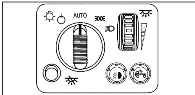
The exterior lamp control is located on the instrument panel on the left side of the steering wheel.
