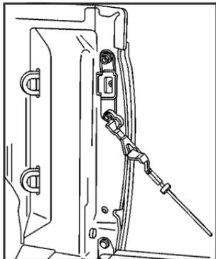
2. Remove the retaining cables from both sides of the tailgate by pulling the clips away from the bolt heads while pushing the cable bracket forward. When the larger part of the hole on the bracket is over the bolt, slide the bracket off of the bolt.
