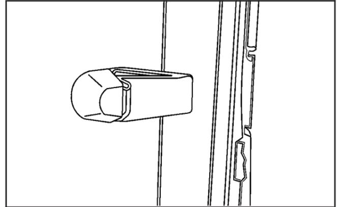
If the vehicle has this feature, squeeze the latch in the center of the window and slide the glass to open it. Be sure the latch is engaged when the window is closed.
