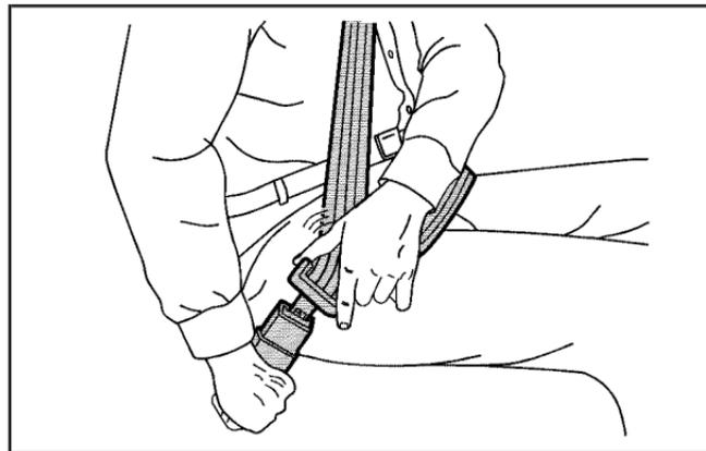
3. Push the latch plate into the buckle until it clicks. Pull up on the latch plate to make sure it is secure. If the belt is not long enough, see *Safety Belt Extender* on page 1-34. Position the release button on the buckle so that the safety belt could be quickly unbuckled if necessary.
