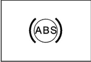
The Antilock Brake System (ABS) light comes on briefly when the engine is started.
