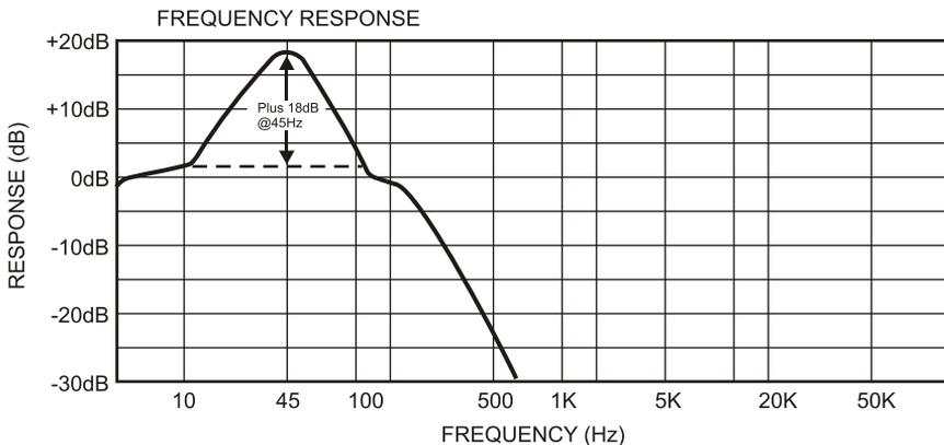
The BASS BOOST control raises the amplifier output up to 18dB at frequencies tightly centered around 45Hz. This "bump" can have a dramatic affect on the bass system's apparent volume. Use caution(!) When adjusting this control as serious subwoofer damage may result from overpowering or overexcursion.
