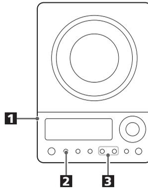
**1** Connect the PHONES jack (audio output jack) of a portable audio player to the AUX IN jack of the CD-X10i using the supplied stereo mini plug cable.
