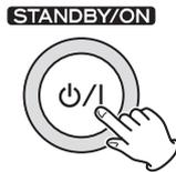
The ring surrounding the STANDBY/ON button lights when the unit is on.
