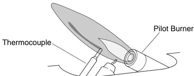
**Figure 22 - Correct Pilot Flame Pattern**
