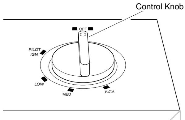
Figure 19 - Control Knob In The OFF Position
