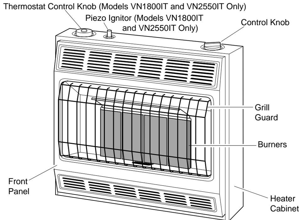
**Figure 1 - Vent-Free Natural Gas Heater (Model VN2550IT Shown)**
