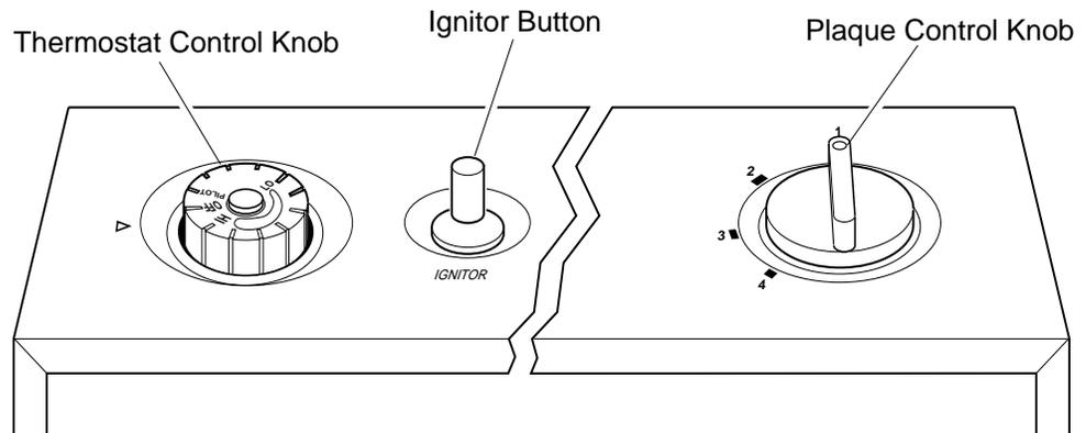
Figure 16 - Thermostat Control Knob In The OFF Position
