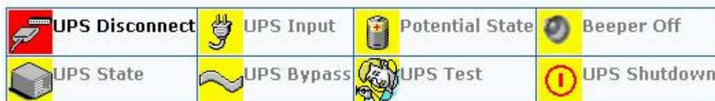
The figure represents the UPS status, when the status has been detected, the figure color change from yellow to red and the status description will changed.
