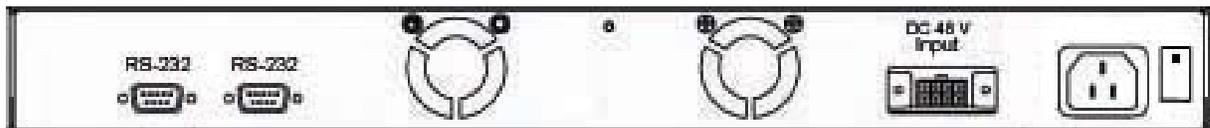
The rear panel of 24 10/100TX plus 2 SFP/Copper managed POE switch
