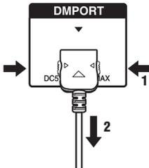
Press and hold both sides of the connector and then pull out the connector.
