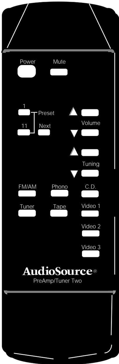
**Power :** Press this button to Turn "ON" the A.C. power to the PreAmp/Tuner Two.
