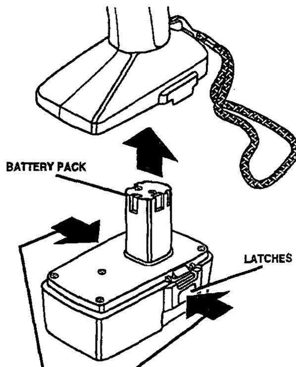
DEPRESS LATCHES TO RELEASE BATTERY PACK
