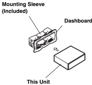
Remove the Detachable Front Panel (refer to page 6). Slide mounting sleeve from main unit (see "Removal" on page 23).
