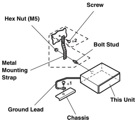
Reinforce the head unit with the metal mounting strap (not supplied). Secure the ground lead of the unit to a clean metal spot using a screw (\*1) already attached to the vehicle's chassis.
