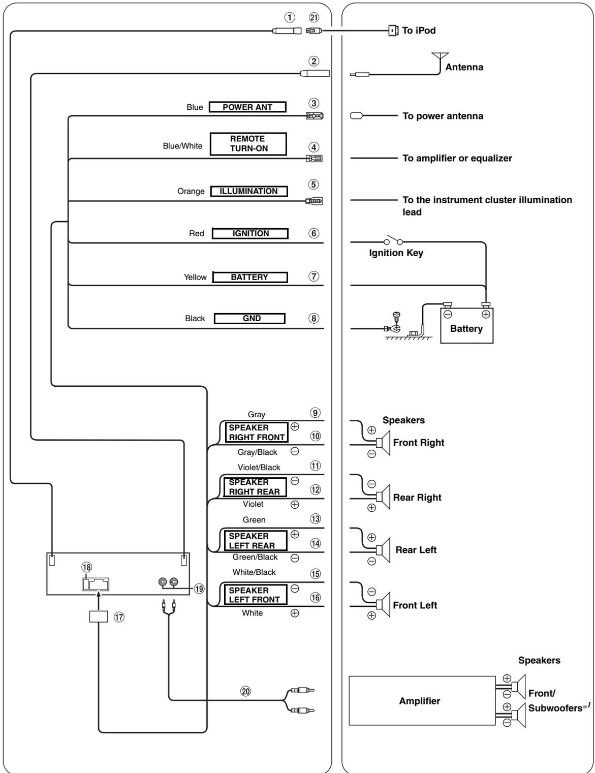
\*1 When Subwoofer is set to OFF :Output is from Front speakers
