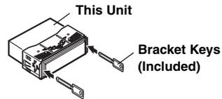
3. Pull the unit out, keeping it unlocked as you do so.
