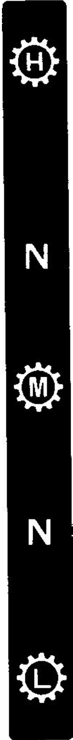
Range Selector Lever - Manual PART NO. - 5BA-390171890 LOCATION - Centre of L. H. fender
