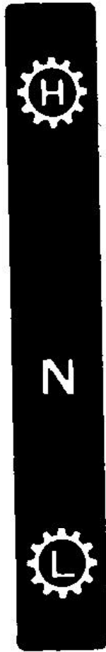
Range Selector Lever - Hydrostatic PART NO. - SBA-39017190Q LOCATION - Centre of L. H. fender
