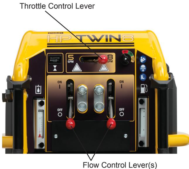
1. Install a calibrated flow and pressure tester across the two hose ends (where the tool would normally be connected).
