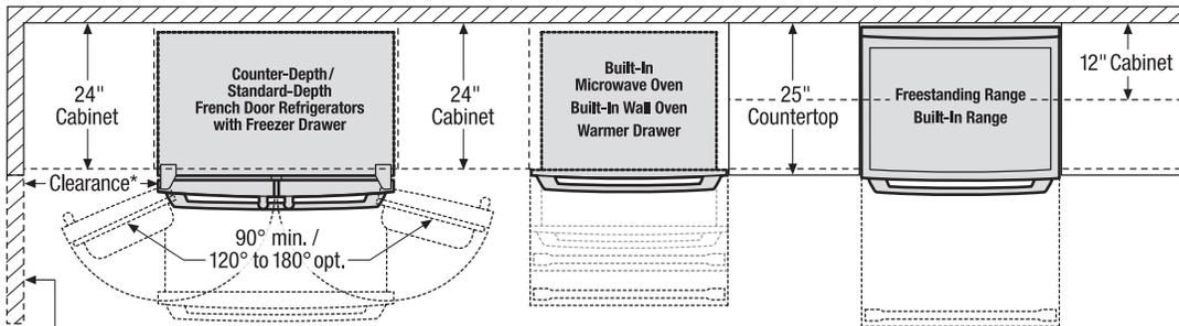
\*When installing a French door refrigerator adjacent to wall, cabinet or another appliance that extends beyond front edge of unit, 20" minimum clearance recommended to allow for optimum 120° to 180° door swing, providing complete drawer / crispener access and removal. (Absolute 4-1/2" minimum clearance will ONLY allow for 90° door swing which will provide limited drawer / crispener access with restricted removal.)
