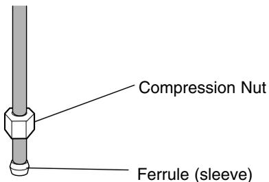
4. Insert the tube into the valve and fasten with wrench as shown in the figure below.
