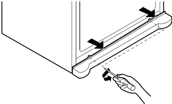
2. Turn the leveling screw clockwise to raise that side of the refrigerator or counterclockwise to lower it. It may take several turns of the leveling screw to adjust the tilt of the refrigerator.
