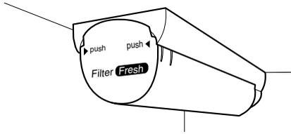
After changing the water filter cartridge, reset the water filter status display and indicator light by pressing and holding the button for 3 seconds.
