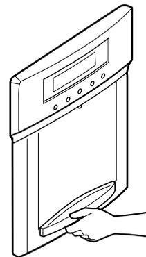
Tilt up the front of tray slightly and snap the ribs into the holes to replace the tray.
