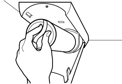
If you can't turn the filter from side to side, it isn't fully inserted. Push it in firmly and use its handle to twist the cartridge clockwise about 1/4 turn. You will hear a snap when it clicks into place.
