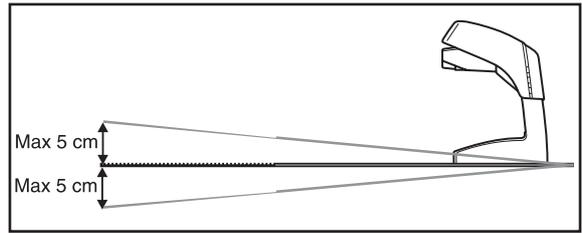
The charging station must not be positioned so that its plate bends.
